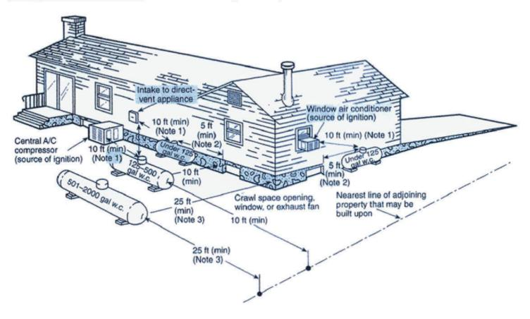
Note: When the cylinder is filled on site from a bulk truck, the filling connection valve and vent valve must be at least 10 feet from any exterior source of ignition, opening into direct-vent appliances, or mechanical ventilation intakes.
